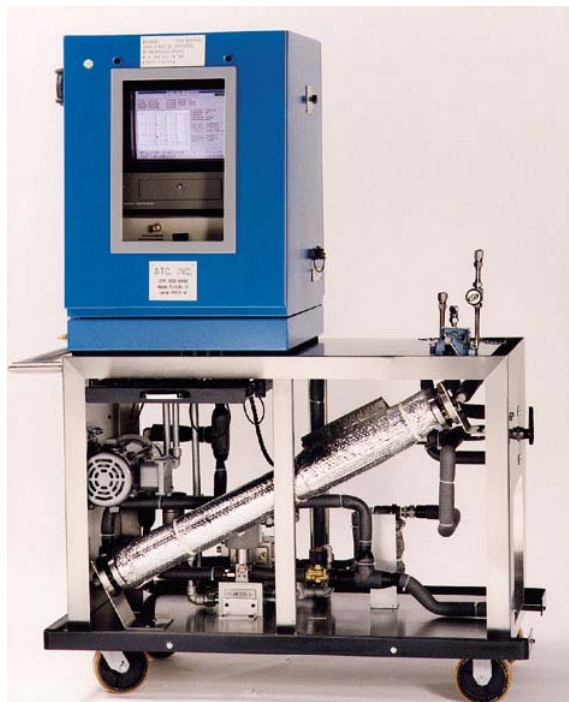
Figure 2: FLO-CAL Cart for Low Flow with Density Standard and Hazardous Environment
